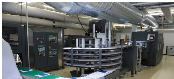
The automated TecnaU Libra 800 makes perfect bound books and brochures, often in different sizes and with a different number of pages from one copy to the next. This is where products pass through the cooling tower before being fed to the Libra VT variable three-knife trimmer (right).
